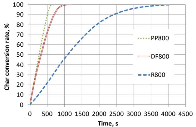
Figure 5. Conversion rate *versus* time for the char sample gasification tests at 850 °C.
