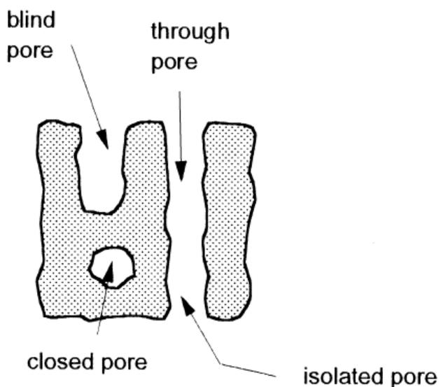
Figure 8. Different types of pores (Leofanti *et al.* 1998).
