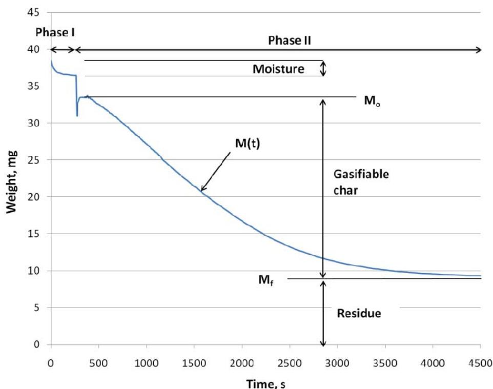
Figure 1. A typical weight loss curve observed during a HPTGA (high-pressure thermogravimetric apparatus) determination of char reactivity.  $M_0$  is the initial mass of char,  $M(t)$  is the mass of char at time  $t$ , and  $M_f$  is the mass of the residue.
