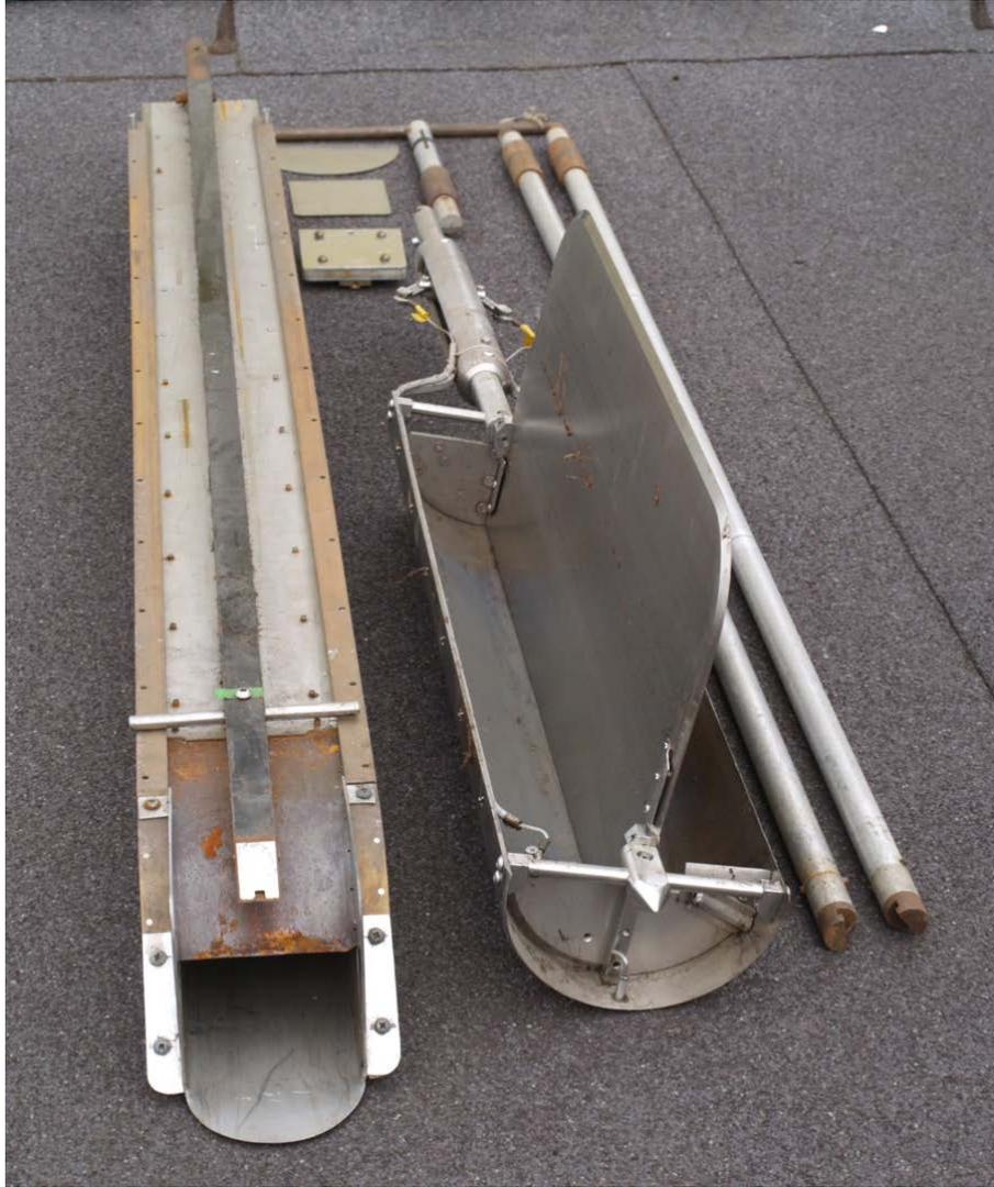
Figure 1. Box corer (left, partly closed) and 'D' corer (right) used in this work. Centre top is the 'T' handle that attaches to extension rods (far right) by 'hand clasp' connections (bottom right). At top is a half-circle divider used for separating samples in the 'D' corer. Below it is a 10 cm square divider used for separating samples in the box corer. Below that is the watertight lowest stopper for the box corer.
