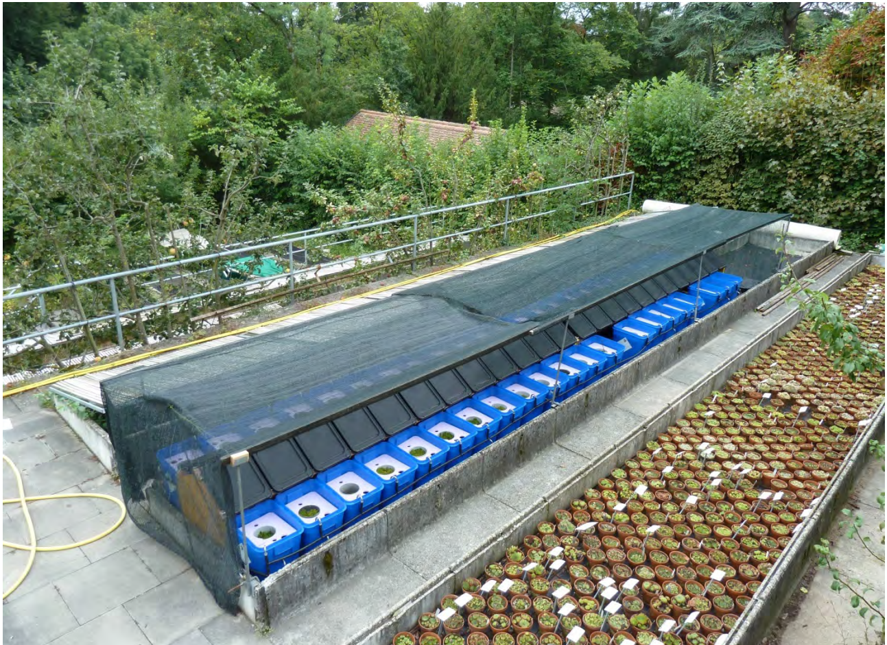
Figure 1. General view of the experimental site, with the 45 mesocosms installed in two rows. Each mesocosm consists of a blue tank, which houses a PVC tube containing a peat core covered by a Sphagnum fallax layer. Each tank has a Styrofoam board cover (with a hole) to prevent direct insolation of the wall of the PVC tube. The (black) lid of the tank is used to increase the amount of water supplied by rainfall. The whole experimental area is fitted with a net that filters out 50 % of the solar radiation; here, the north-facing part of the net has been removed for display purposes.
