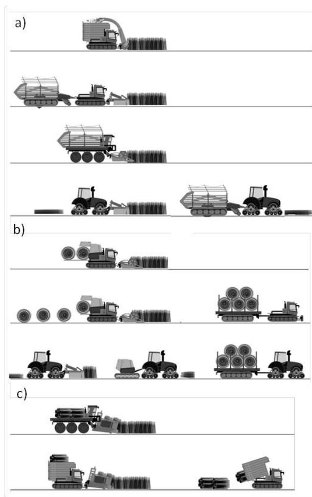
Figure 6. Examples of different approaches to biomass harvesting in wet peatlands. The biomass is: a) chopped or cut; b) baled; or c) bundled. Depending of the position of the water table, it is harvested in one, two or three working steps. If the biomass is dried on the ground, further steps such as tedding and swathing (i.e. arranging and reworking the cut harvest so as to promote drying) may be added.
