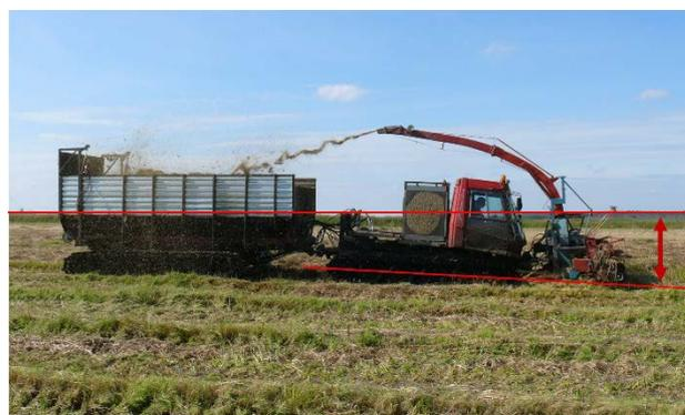
Figure 2. An example of vehicle being off-balance due to harvesting equipment attached at the front. Photo: S. Wichmann (2011), Murchiner Wiesen, Mecklenburg - Western Pomerania, Germany.
