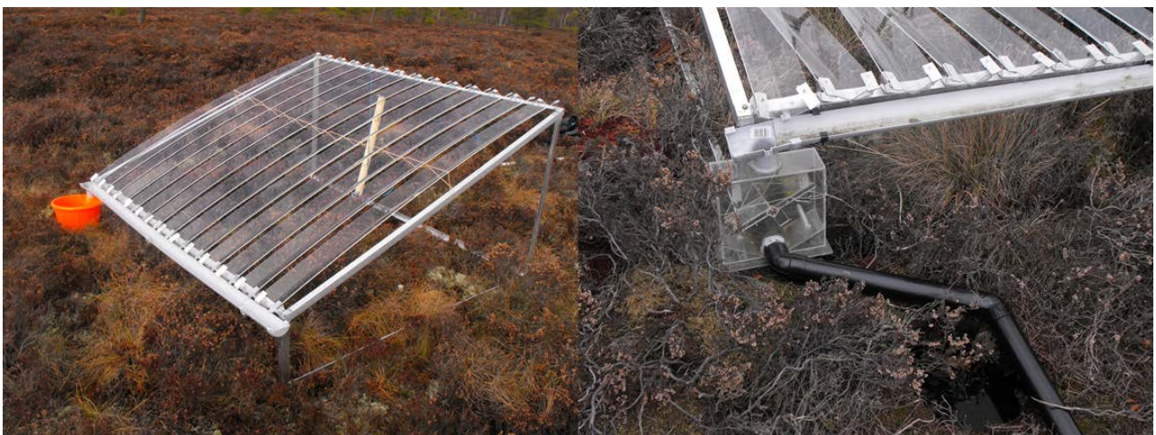
Figure 1. Design of the rainfall shelters showing the arrangement of the roof drainage system
