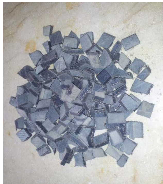
Figure 3. Shredded tyre chips. The dimensions of each chip are 20 \times 15 \times 0.5 mm.
