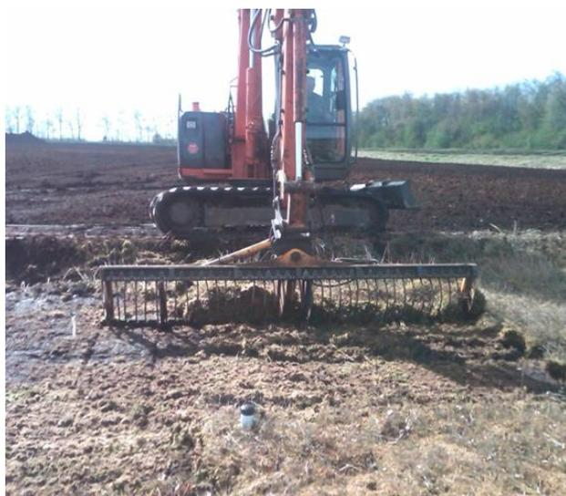
Figure 2. Excavator with mowing basket harvesting *Sphagnum* on the Ramsloh Test Field, October 2015.
