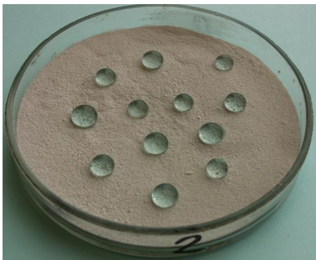
Figure 4. Petri dish containing modified gypsum powder, with drops of water applied to the surface.
