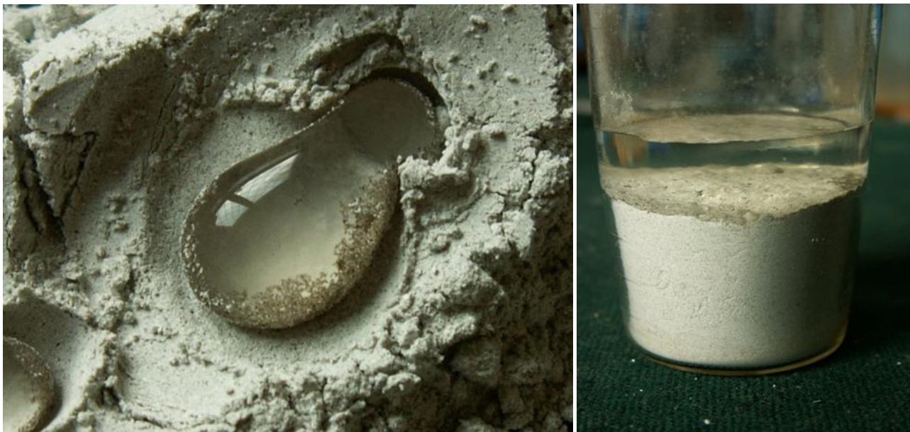
Figure 3. Options for preliminary tests of the hydrophobicity of modified gypsum binder.
