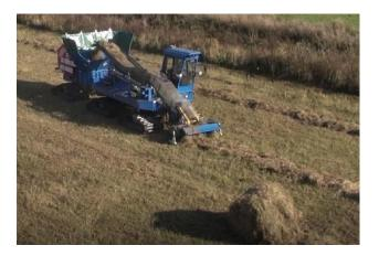
Figure 3. The tracked vehicle units designed by PIMR for non-stop swath collecting and forming bales. Photo: PIMR archive.
