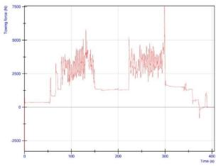
Figure 7. Above: the Prowler being used as a mini tractor for the biomass train in the field trials near Biala in October 2015. Photo: PIMR archive. Left: The forces on the clevis pin hitch when towing five biomass bales during the October 2015 field trials (NI 2012).
