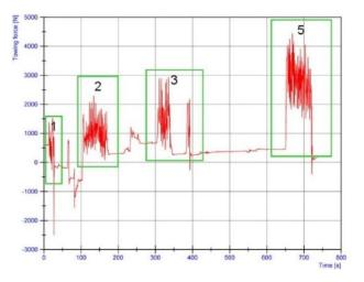
Figure 6. Towing forces for 1, 2, 3 and 5 biomass bales measured during the biomass train field trials at the Byszewice site (NI 2012).
