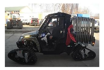
Figure 4. Prowler 700HDX rebuilt into a tracked mini tractor for biomass trains. Note the (red) mud shoes hanging on back of cab. Photo: PIMR archive.
