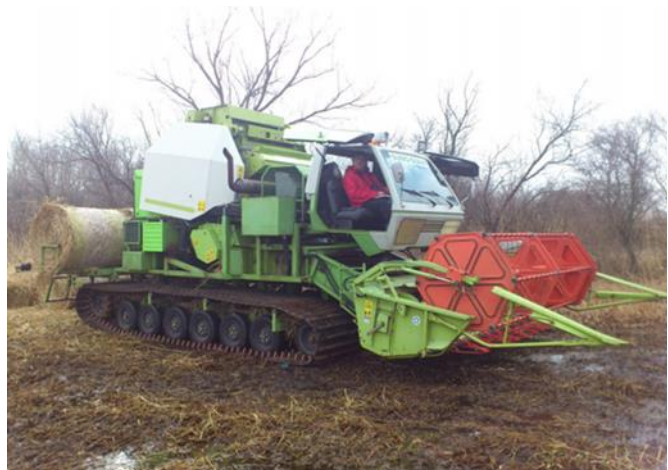
Figure 4. Examples of specialised wetland harvesters from Europe. Left: the tracked wetland harvester Pisten Bully GreenTech 100 (left) manufactured by Kässbohrer (source: http://www.offpisteagri.co.uk/pictures-worth-seeing.html ). Right: the Sumo -Quaxi Machine from Austria that cuts and bales (source: http://duene-greifswald.de/doc/rrr2013/talks/Harvesting%20Techniques%202_Beckmann%202013%20-%20Harvesting%20Technologies%20for%20reeds%20in%20Austria.pdf ).
