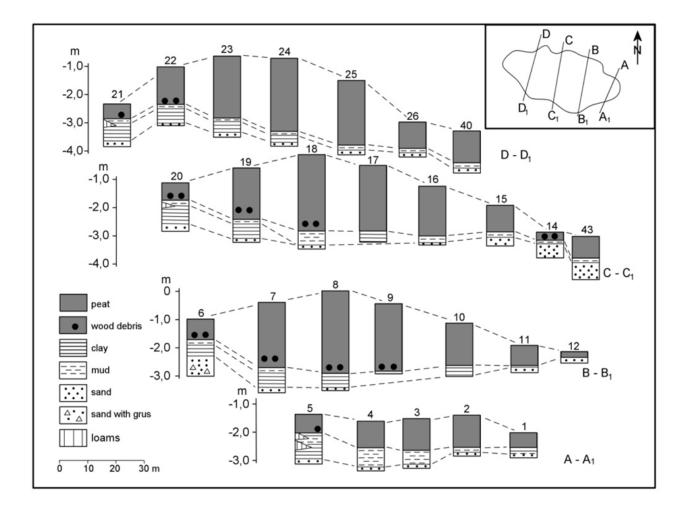
Figure 6. Lithology of alluvium in the substrate of the Łokieć bog along four transverse sections. Locations of cross-section lines and borehole numbers as in Figure 2.
