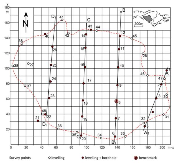
Figure 2. Network of levelling points and boreholes at the Łokieć bog.
