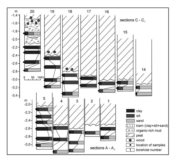
Figure 7. Grain-size distribution beneath the Łokieć bog. Numbers of cross sections and boreholes as in Figure 2.
