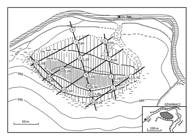
Figure 4. Network of boreholes (1-15) on the Dźwiniacz bog with interpolated depth of the peat base (contours: 1 m, 2 m).
