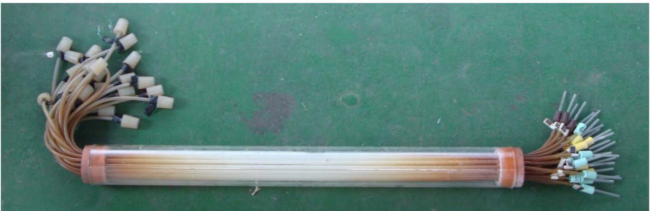
Figure 6. Multiple air-cooled condenser used to collect water (including tritium) after heating peat/clay in an oil bath at 130 °C in tubes attached by the silicone rubber bungs to the left. In use the condenser sloped downwards (left to right) to the collecting test tubes, shielded by the plastic caps at the right.
