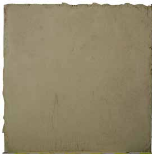
Figure 16. Sample 7: finished clay plaster.
