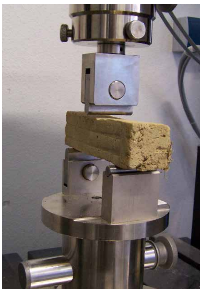
Figure 7. The bending tensile strength test (left) and the pressure strength test (right).
