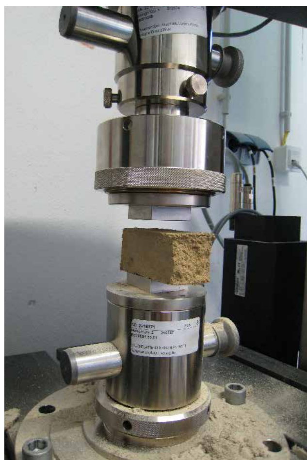
Figure 7. The bending tensile strength test (left) and the pressure strength test (right).
