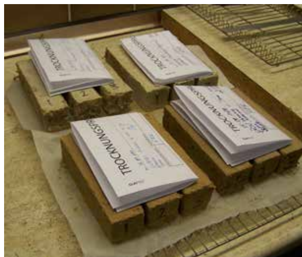
Figure 6. Test specimens after 28 days of dehydration in the climate chamber.
