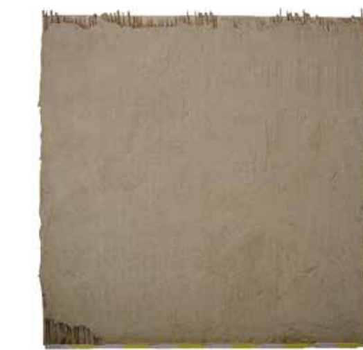
Figure 14. Sample 6: dry finished clay plaster.
