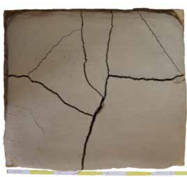
Figure 8. Sample 1 (not reinforced) developed deep and spreading structural cracks during drying.
