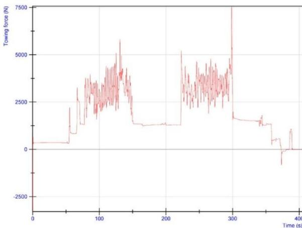
Figure 7. Above: the Prowler being used as a mini tractor for the biomass train in the field trials near Biala in October 2015. Photo: PIMR archive. Left: The forces on the clevis pin hitch when towing five biomass bales during the October 2015 field trials (NI 2012).
