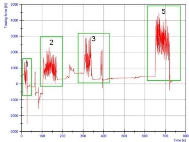
Figure 6. Towing forces for 1, 2, 3 and 5 biomass bales measured during the biomass train field trials at the Byszewice site (NI 2012).
