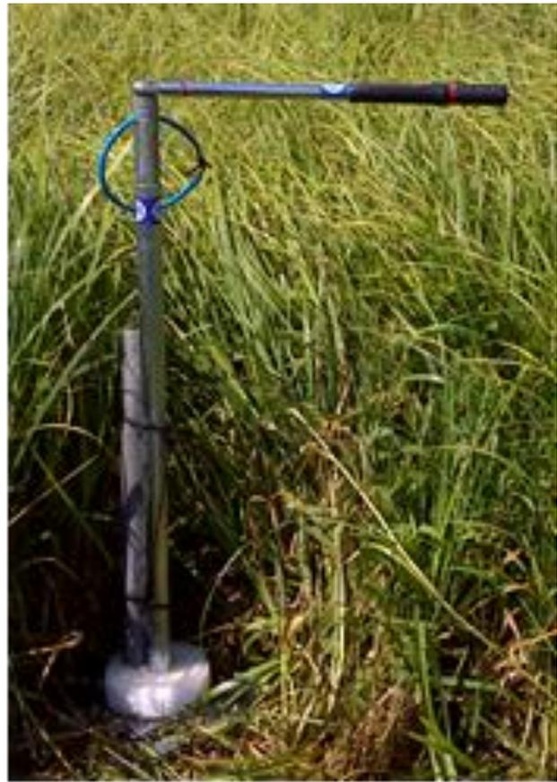
Figure 1. Using a portable spiked plate (made by PIMR) with torque wrench to test surface strength in a sward of common reed on organic muck soil, water table depth 0.5 m. Photo: PIMR archive.
