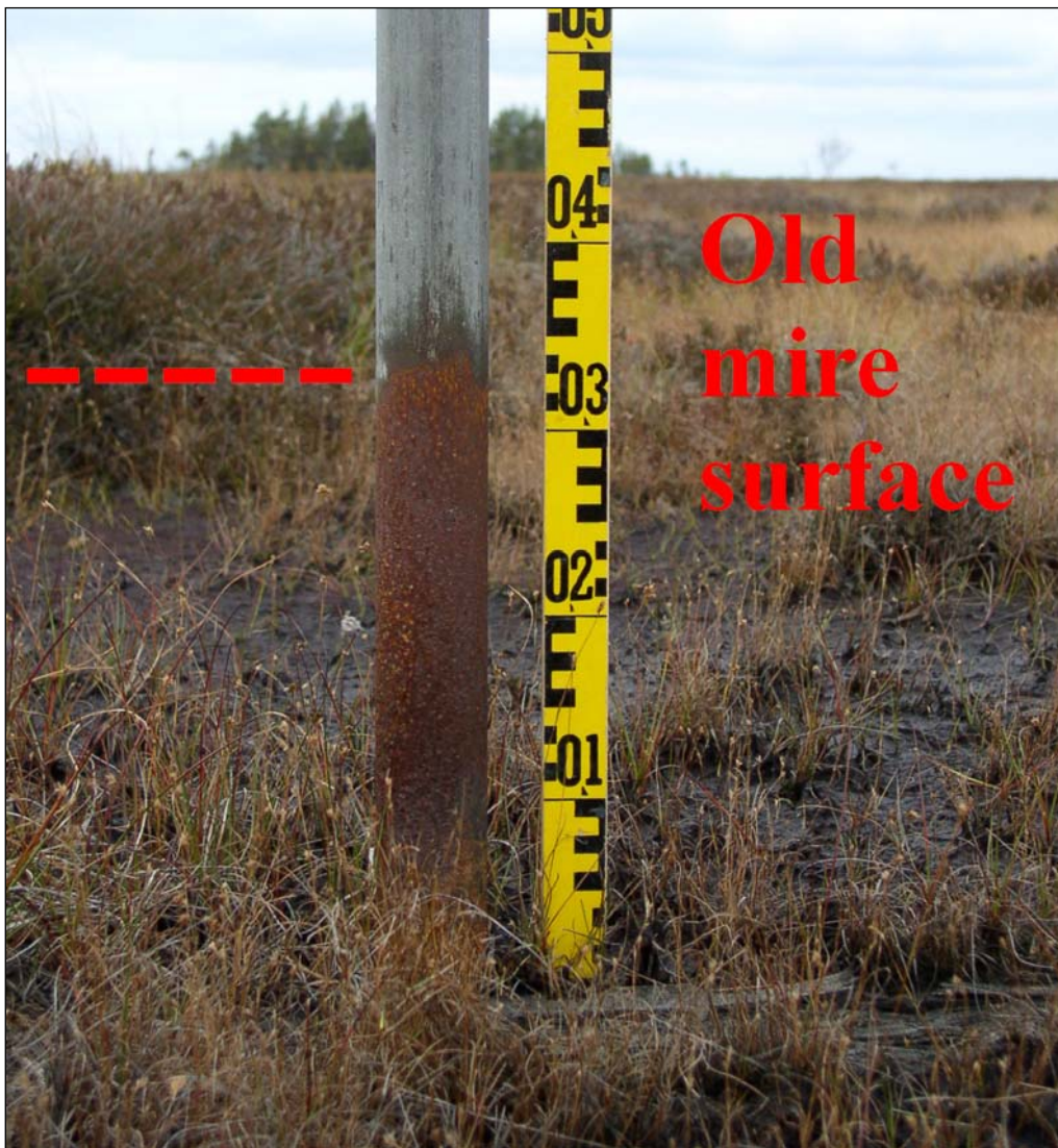
Plate 5. Close view of the IHD steel tube shown in Plate 4, at Björnsjömossen (Site 6 in Figure 2) in the Komosse Bog Complex. The sharp boundary between corroded and non-corroded tube galvanization shows the former position of the bog surface, and the length of the rusty section gives a rough indication of the amount of subsidence that has occurred since 1970.
