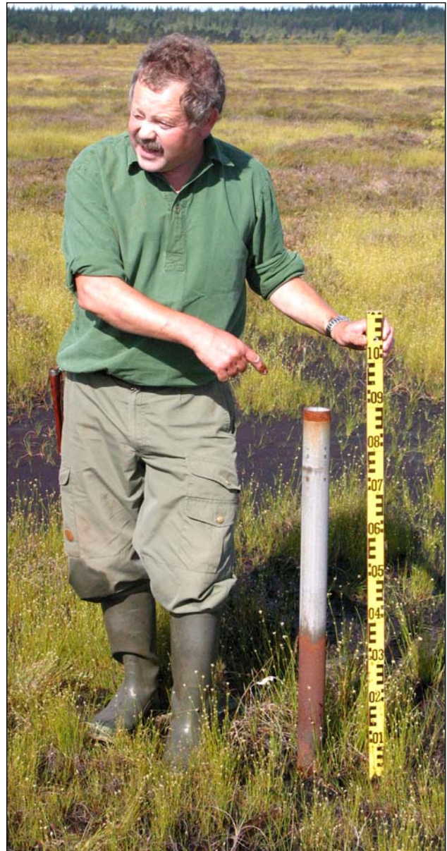
Plate 4. Demonstration of the measurement procedure for the IHD steel tubes on the Komosse Bog Complex. This and all the other IHD tubes were visited and re-measured five times between 1996 and 2005.
