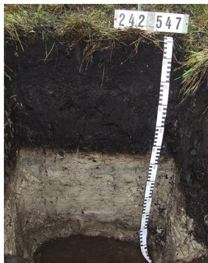
Figure 4. Typical soil profile for a drained terrestrialisation mire, consisting of peat over calcareous gyttia.
