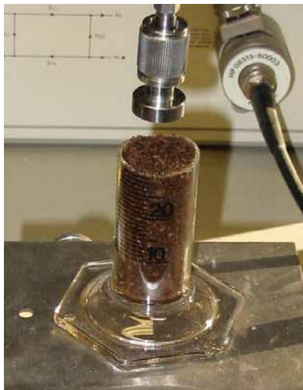
Figure 2. A newly-filled sample holder prior to a typical permittivity measurement.
