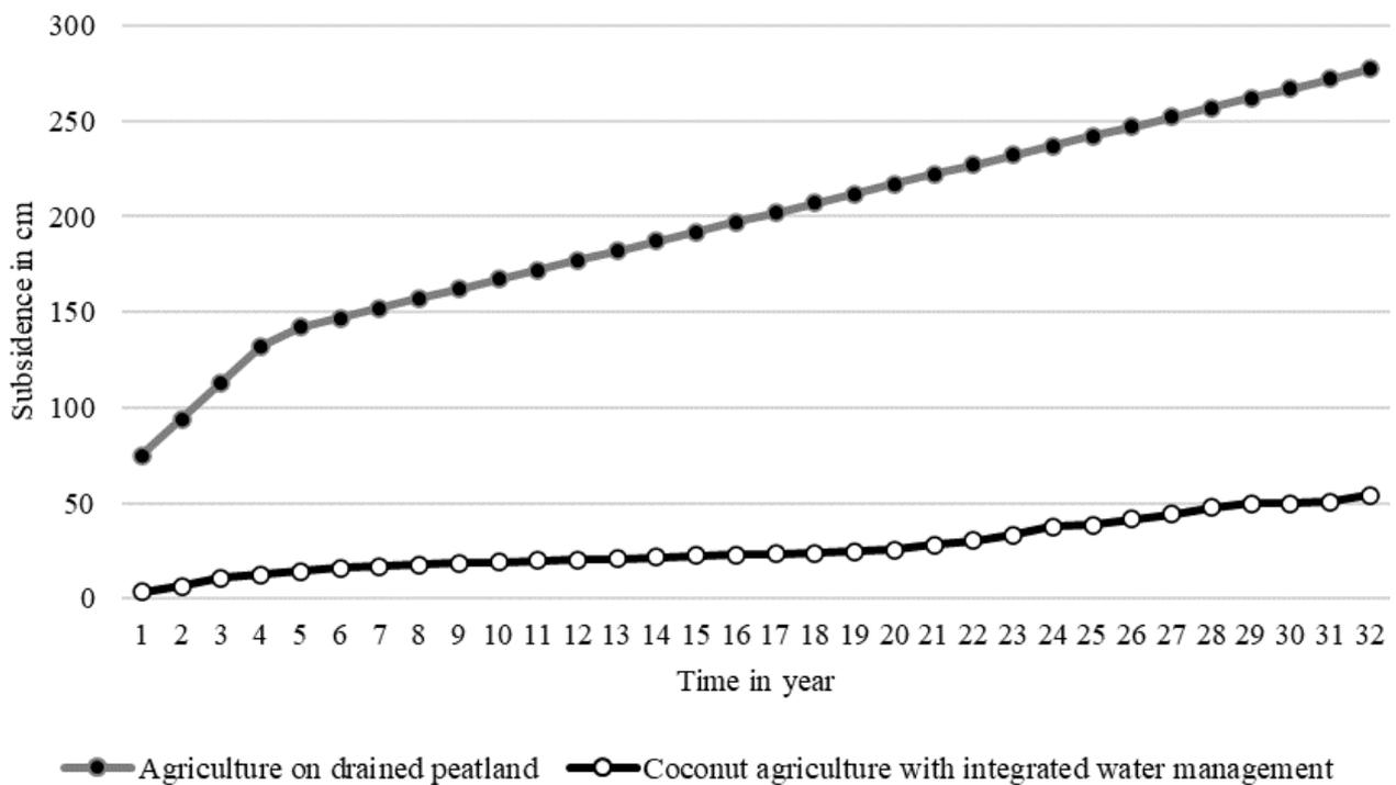
Figure 5. Comparison of accumulated subsidence between drained peatland under agriculture from Hooijer *et al.* (2012), and the Pulau Burung coconut plantation area.
