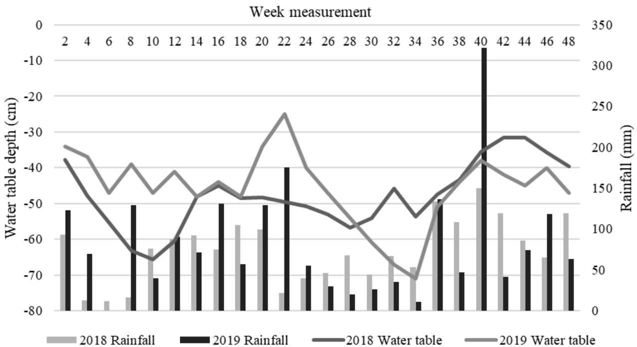
Figure 4. The average water table depth from measurement data collected at 106 points, alongside rainfall data in the study area.
