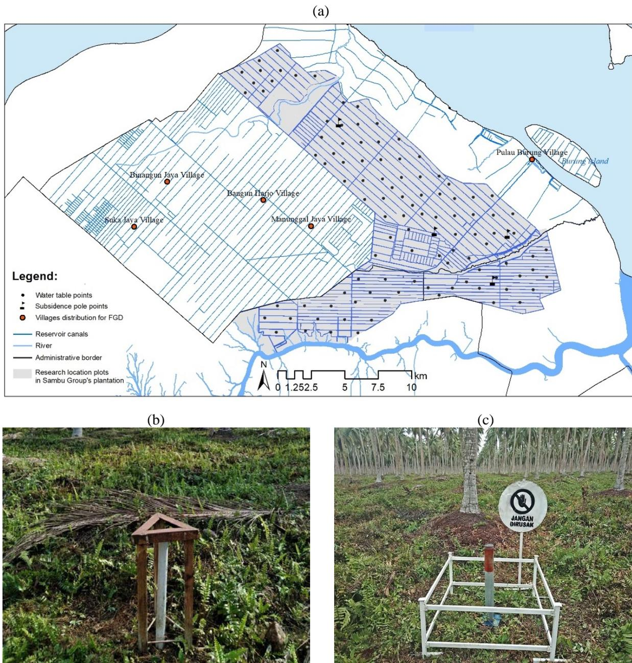
Figure 3. (a) Map showing the distribution of water table and subsidence measurement points in the Sambu Group plantation, and the locations of the five FGD villages. (b) PVC tube for measurement of water table level. (c) Iron pole for subsidence measurements.
