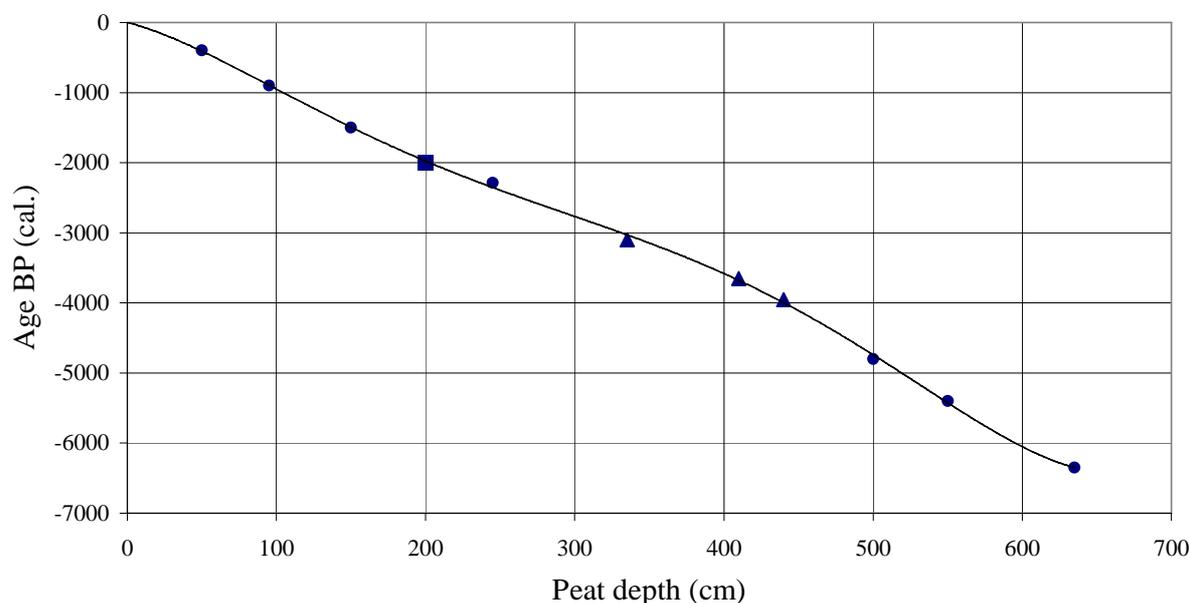
Figure 9. Datings from Lyngmossen, south-west Sweden. Dots are  $^{14}\text{C}$ -datings, triangles are tephra horizons and the square is the Antique high peak of the Pb curve (dates are given with negative values for drafting reasons). A sixth-order polynomial fitted to these data was used to calculate age for various depths.
