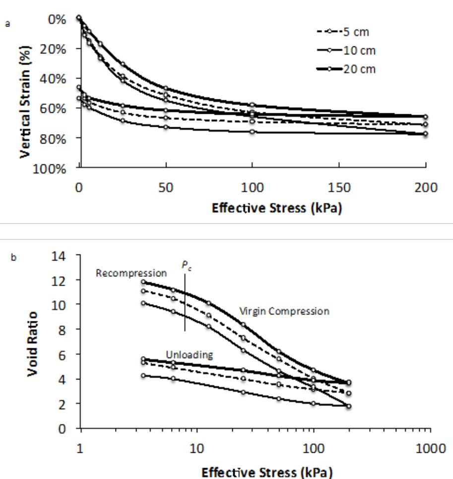
Figure 4. Loading and unloading curves for gyttja showing (a) strain and (b) void ratio, both *versus* log-scale effective stress.
