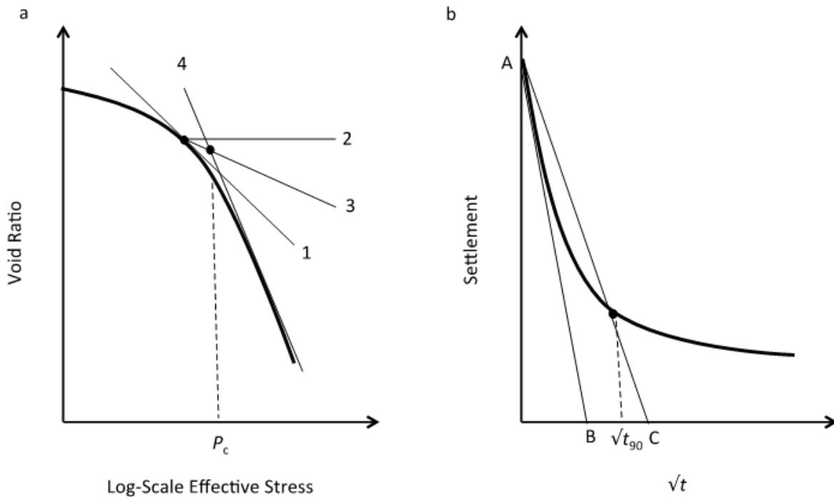
Figure 1. Graphical procedures for estimating (a) preconsolidation pressure following Casagrande (1936), and (b) time of 90 % consolidation following Taylor (1948). See text for details.
