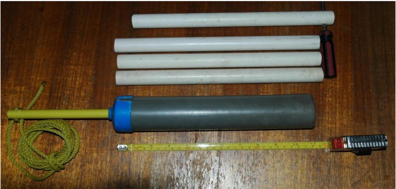
Figure 3. Corer used for sampling smaller and softer aestivation site deposits.
