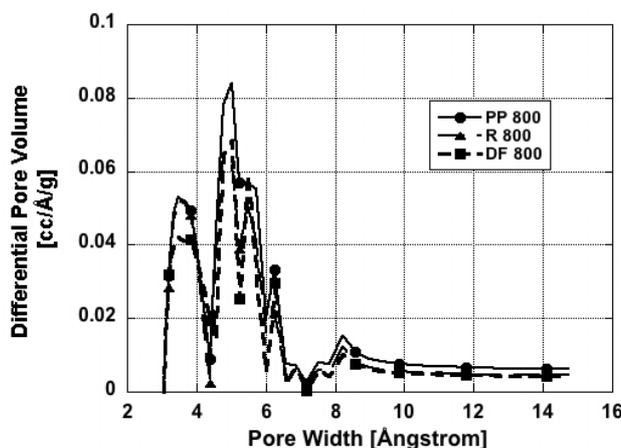
Figure 3. DFT/Monte-Carlo differential pore volume distribution. DFT Kernel used: CO<sub>2</sub> at 0 °C on carbon.
