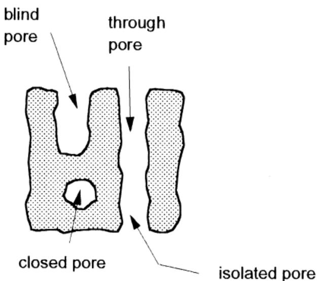
Figure 8. Different types of pores (Leofanti *et al.* 1998).
