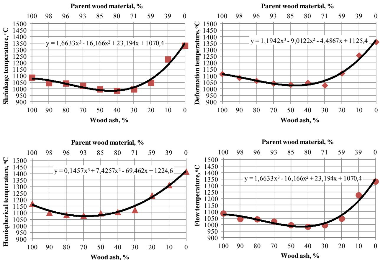
Figure 6. Plots of ash fusion temperature data for blends of wood and reed (see also Table 6).
