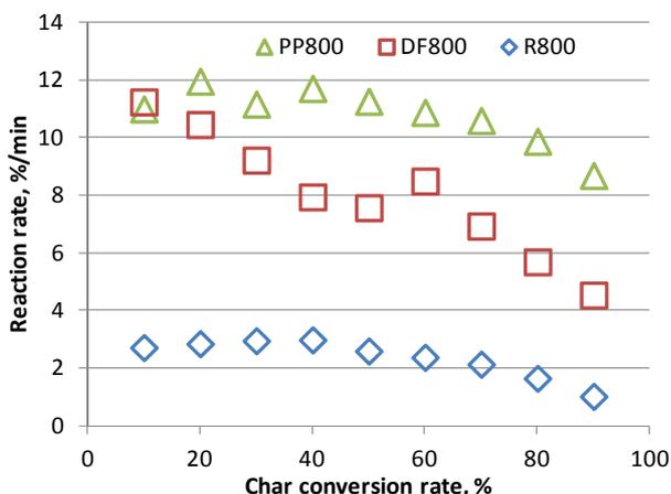
Figure 4. Reactivity of the char samples during the course of gasification at 850 °C.
