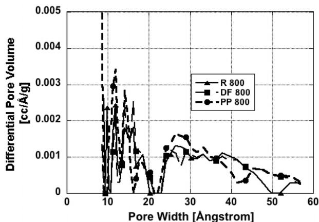
Figure 2. DFT/Monte-Carlo differential pore volume distribution. DFT Kernel used: N<sub>2</sub> at -196 °C on carbon.
