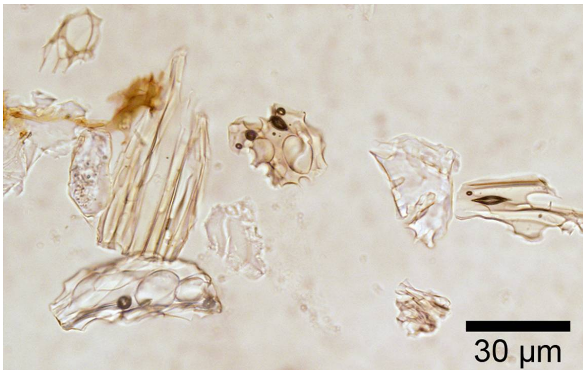
Figure 1. Photograph showing tephra shards with characteristic fluted and vesicular morphologies. The shards are from a currently unidentified tephra layer from the Shetland Isles, UK.
