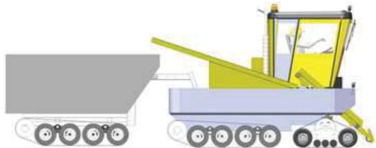
C. Virtual model of an amphibian tracked unit with modified front tracks.
