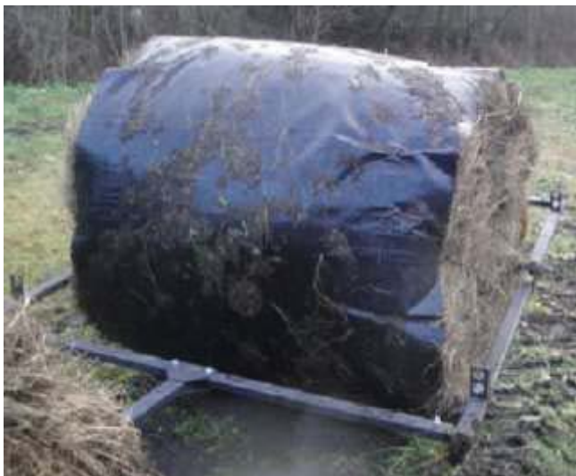
D. Textile cover on a 1.25 m diameter biomass bale after a 1.6 km rolling test on peatland (from Dubowski et al. 2012e). There was no damage to the textile cover.
