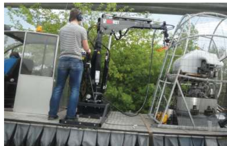
D. The AHTC with equipment for removing bushes and small trees, during a yard test.
