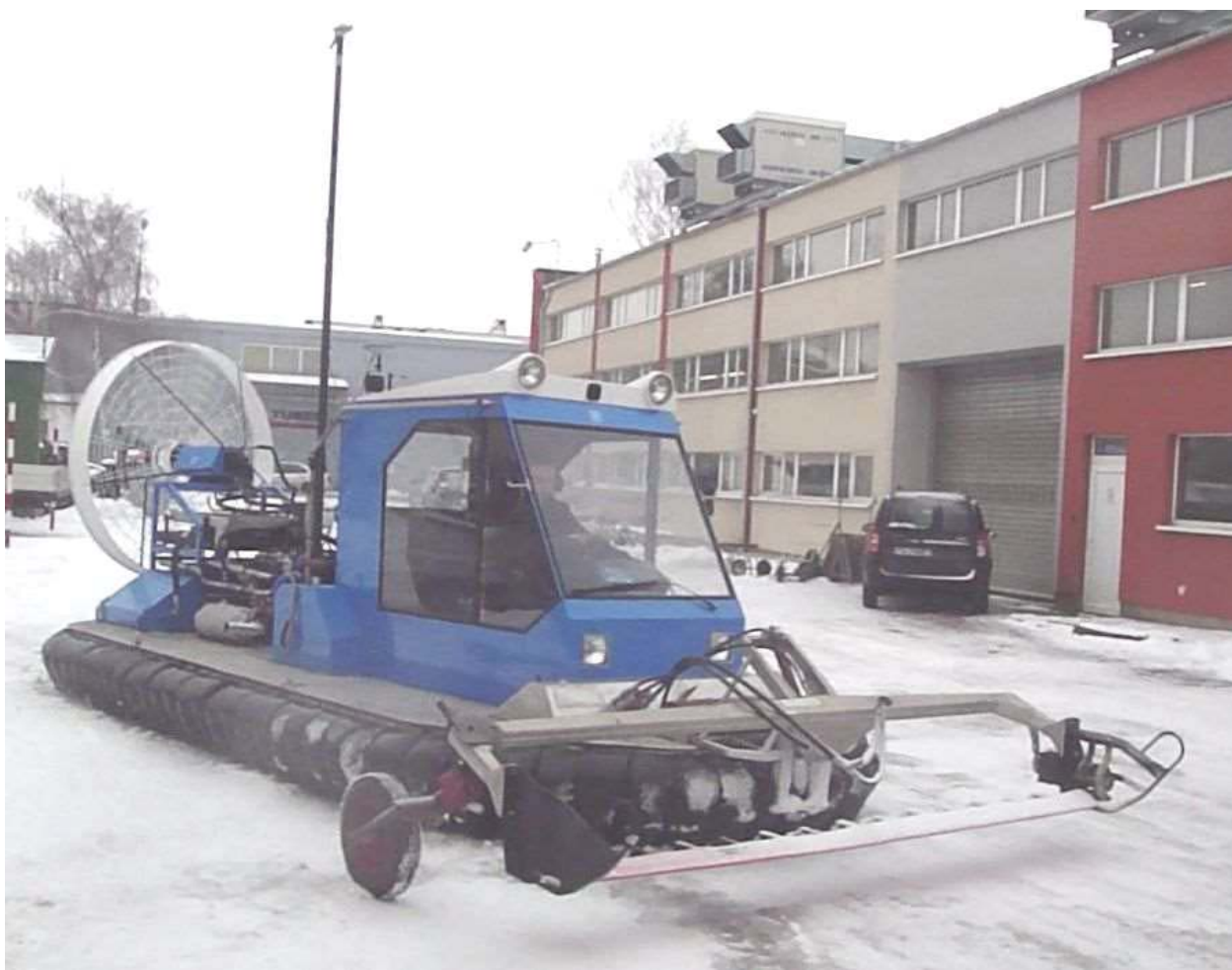
Figure 7. The second prototype AHTC with mower. The mower has been fitted (temporarily) with a wheel to increase driveability during flights over the training area.
