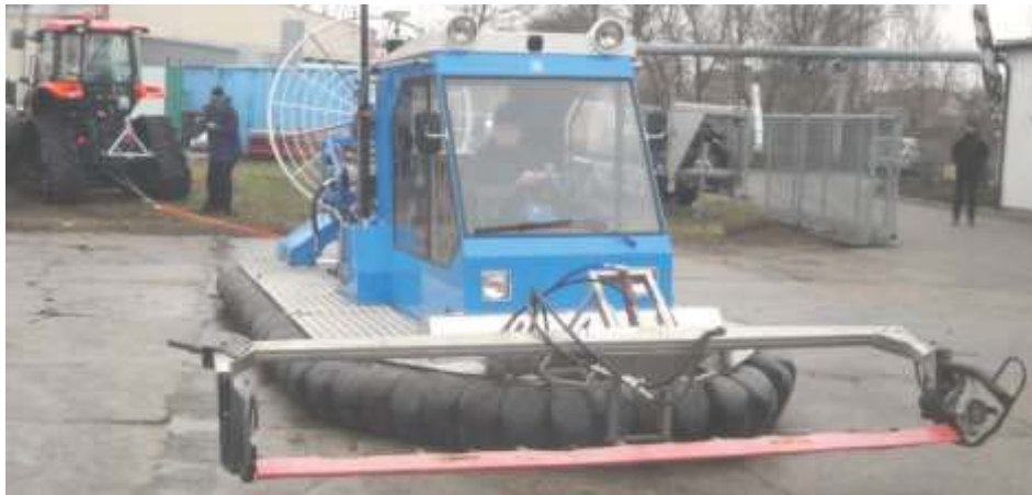
B. The second AHTC prototype undergoing propeller thrust force tests during a flight over a concrete surface. A Kubota tractor is being used as an anchor point for the rope.
