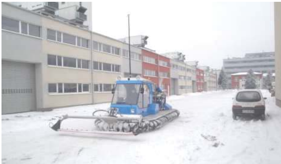
C. The second prototype AHTC during a yard test. The mast is a mounting for HD cameras.
