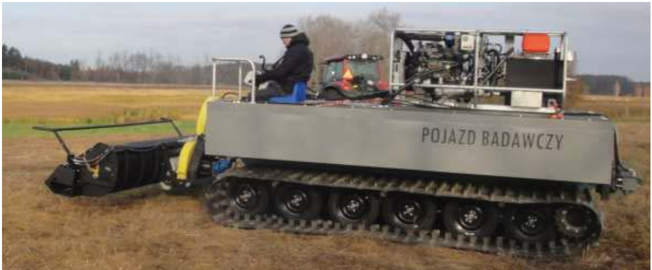
A. The pre-prototype version of the tracked amphibian tractor during field testing.
