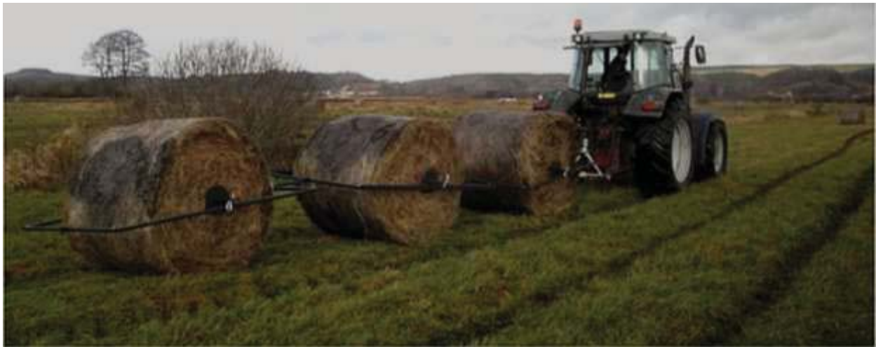
A. A 'biomass bales train' consisting of a farm tractor and three biomass bales (diameter 1.25m).
