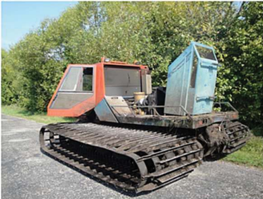
A. Snow groomer with an open engine cover. The build-up of biomass dust on oily surfaces makes this a potential fire hazard.
