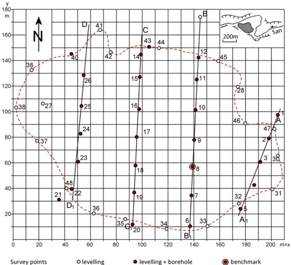
Figure 2. Network of levelling points and boreholes at the Łokieć bog.
