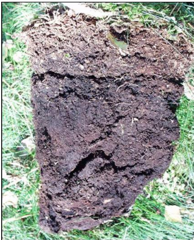
Figure 1. Peat aggregation (crumbs) in the peat shrinkage horizon of a fen.
