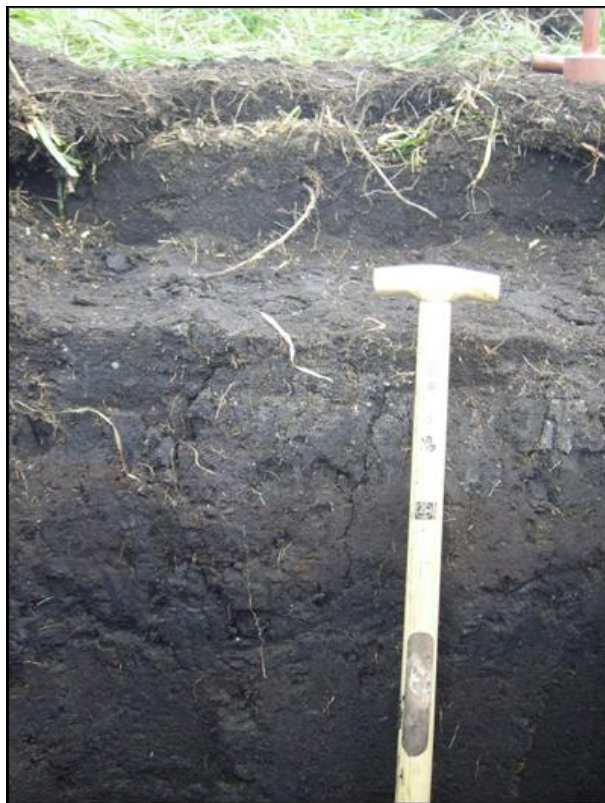
Figure 2. Shrinkage cracks in fen peat due to aerobic conditions associated with agricultural use.
