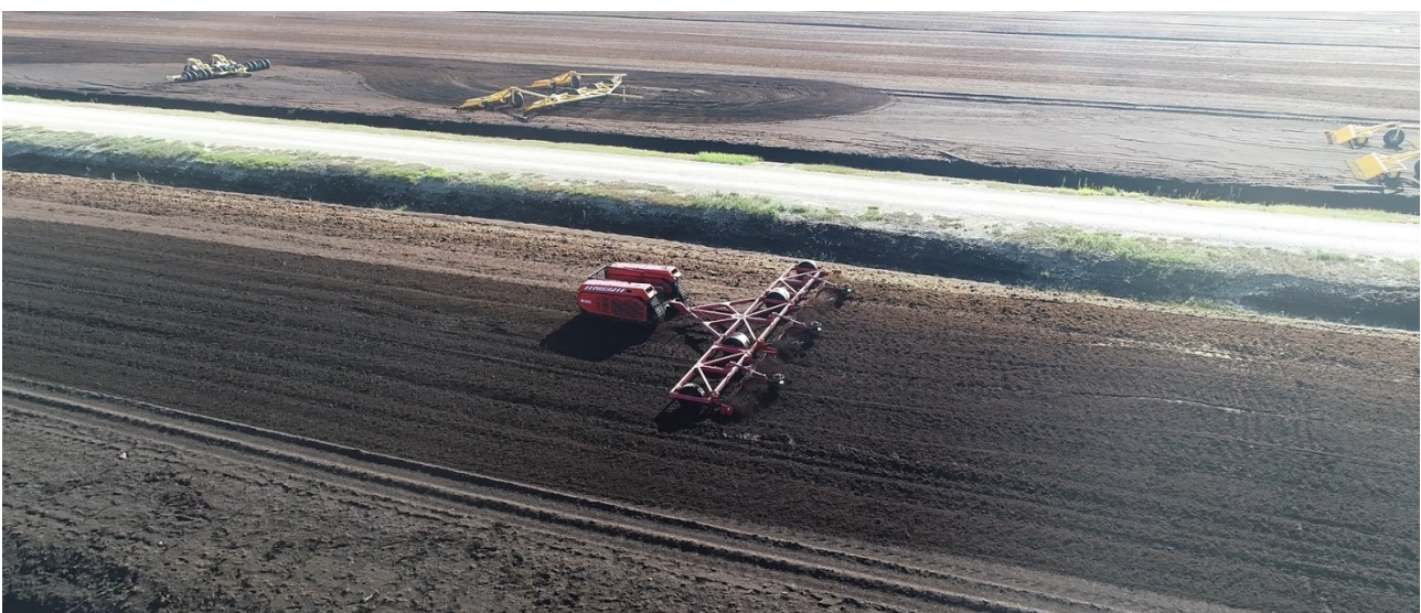
Figure 3. The Multiscope UGV towing a passive miller.
