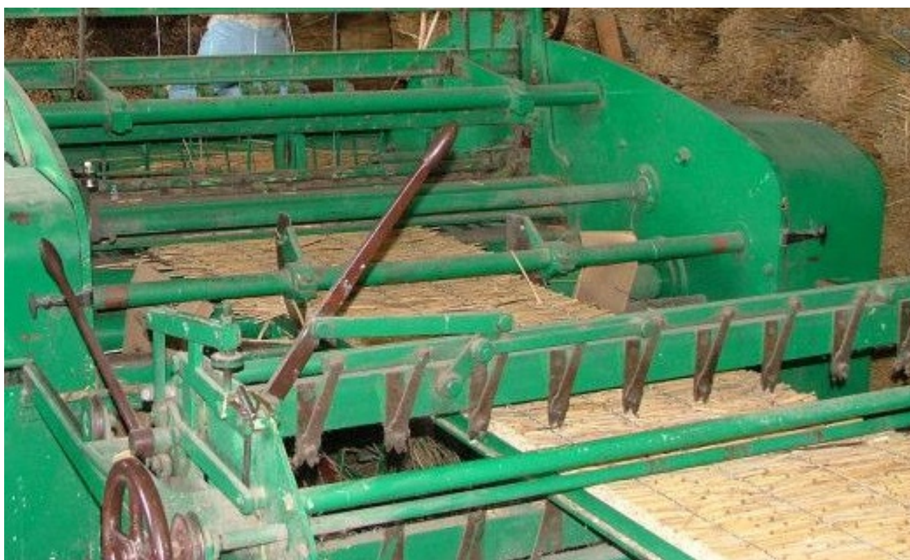
Figure 4. Above: machine from China for making reed boards; below: machine for making Berger boards. Reed boards 50 mm thick, cut to size, were used to fill the recesses between the (50 × 50 mm) supporting timbers of wall type VS2, both inside and outside, thus creating relatively flat surfaces for plastering.
